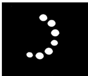
**Figure 1a.** Proton image of seven capillaries filled with (from top to bottom) natural abundance (NA) water, 10%  $\text{H}_2^{17}\text{O}$ , NA, 20%  $\text{H}_2^{17}\text{O}$ , NA, NA, and 40%  $\text{H}_2^{17}\text{O}$ .
