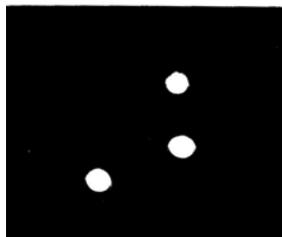
**Figure 1b.** O-17 image of the same set of capillaries shown above. It is seen that only O-17 enriched water is detected (the NA water contains too little O-17 to be seen).
