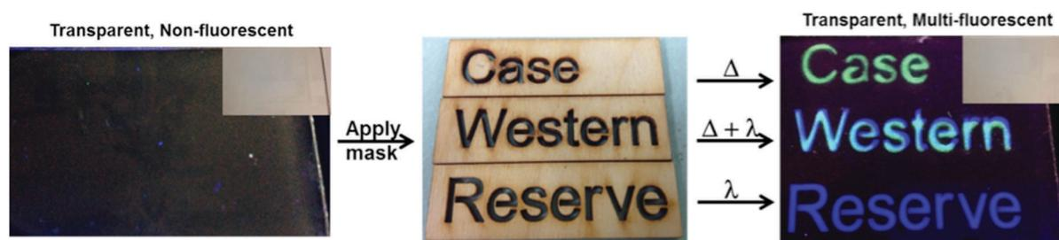
**Fig. 1** Overview of work presented herein: transparent and non-fluorescent PMMA film containing two orthogonally responsive dyes, use of a wooden mask and thermal and photo stimuli to give a transparent film with fluorescent pattern and data storage in 0 (no fluorescence), 1 (green fluorescence), 2 (aquamarine fluorescence), and 3 (blue fluorescence). Polymer film is 3 cm × 5 cm; main image shows film under UV light and insets show full film under ambient light.
