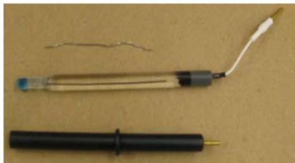
Figure 1. (TOP) Potentiostat (Cypress Systems) and electrochemical cell. (Bottom) Electrodes used in this experiment: (A) Pt counter electrode, (B) Reference electrode, and (C) Pt working electrode.
