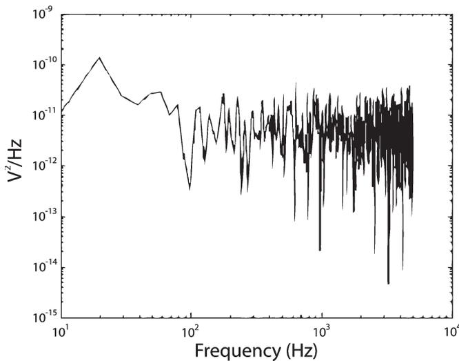
Fig. 12. Measured input-referred noise spectral density of the wireless recording unit.
