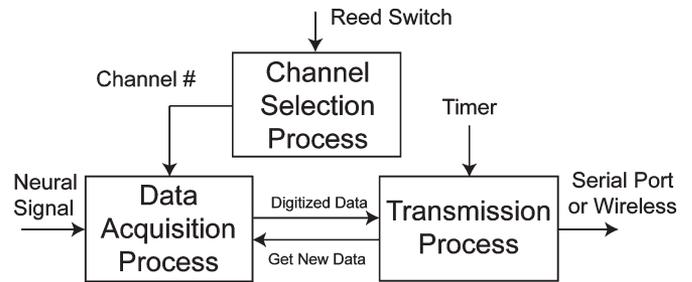
Fig. 7. Block diagram illustrating microcontroller processes in the wireless recording unit.
