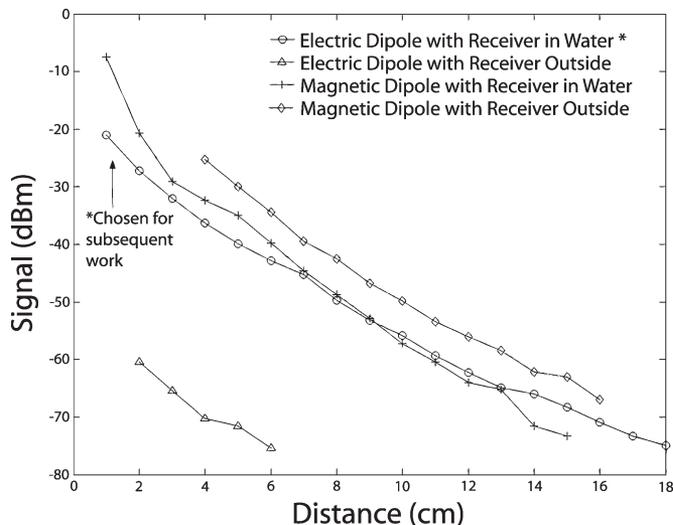
Fig. 4. Measured received signal strength as a function of distance for electric and magnetic-dipole antennas with receive antenna inside and outside water. The transmit signal is supplied by a 0-dBm source.
