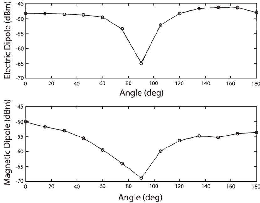
Fig. 5. Measured orientation dependence of electric and magnetic-dipole antennas. Data indicate the received signal strength as function of angle between the two, which is at a distance of 8 cm.
