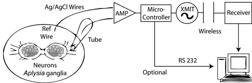
Fig. 10. Experimental setup for *in vitro* neural tests.
