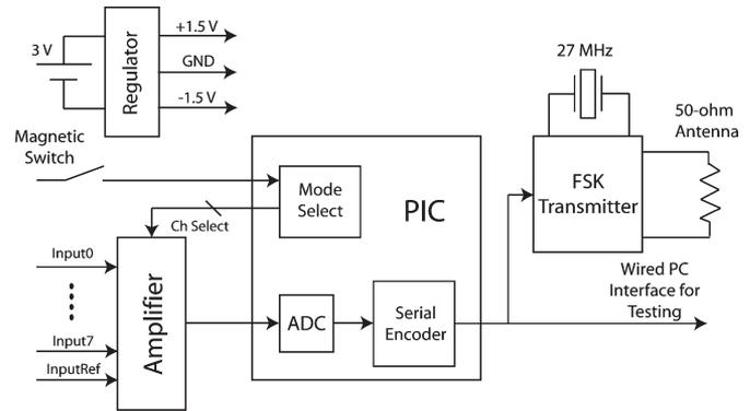
Fig. 2. Overall block diagram of the implantable wireless recording unit.
