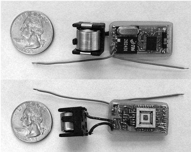
Fig. 11. Photograph of the wireless recording unit.
