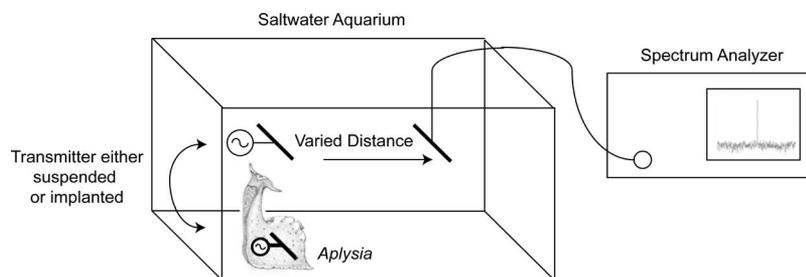
Fig. 3. Experiment setup for antenna testing in an aquarium. Transmitting antenna is either submerged or attached to a moveable pipe or implanted in a live animal (*Aplysia* sketch from [43]).
