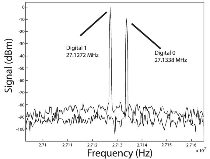
Fig. 17. Measured FSK spectra from the recording unit using antennas in close proximity and constant binary inputs.
