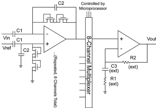
Fig. 6. Schematic of the eight-channel bioamplifier.
