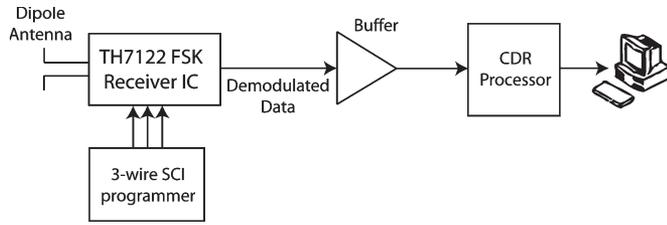
Fig. 8. Block diagram of the 27-MHz FSK receiver including serial control interface (SCI).
