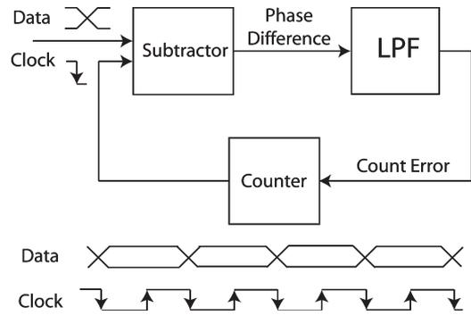
Fig. 9. Block diagram of CDR algorithm used in the receiver microcontroller including low pass filter (LPF).
