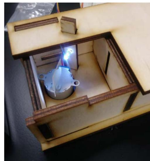
*Above: The illuminating compartment of a simple spectrophotometer that students assemble and test in the instrumentation core laboratory.*
