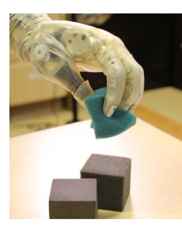
applied between the hand and objects as the hand closes around them. These sensors are connected to a external system that transforms the pressure signals into a neural code that is transported through wires to electrodes that are surgically implanted in the subjects residual arms. When the neural code reaches the nerves, a connection is made between the prosthetic and the brain, which interprets the signals as a sense feeling in the subject's own hand.
