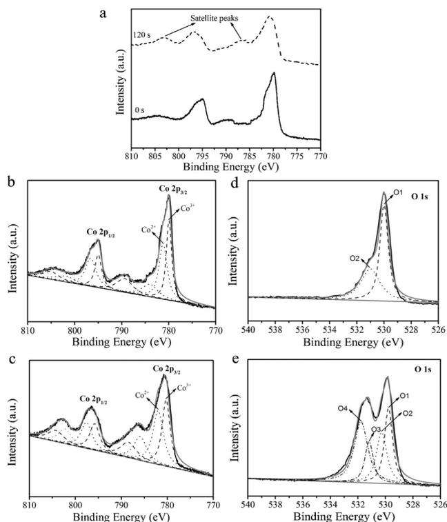
**Figure 3.** a) Co 2p XPS spectra of pristine  $\text{Co}_3\text{O}_4$  and plasma engraved  $\text{Co}_3\text{O}_4$ . b), c) Fitted Co 2p for pristine  $\text{Co}_3\text{O}_4$  (b) and for plasma-engraved  $\text{Co}_3\text{O}_4$  (c). d), e) Fitted O 1s for pristine  $\text{Co}_3\text{O}_4$  (d) and plasma-engraved  $\text{Co}_3\text{O}_4$  (e).
