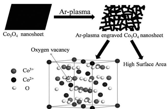
**Scheme 1.** Illustration of the preparation of the Ar-plasma-engraved  $\text{Co}_3\text{O}_4$  with oxygen vacancies and high surface area.
