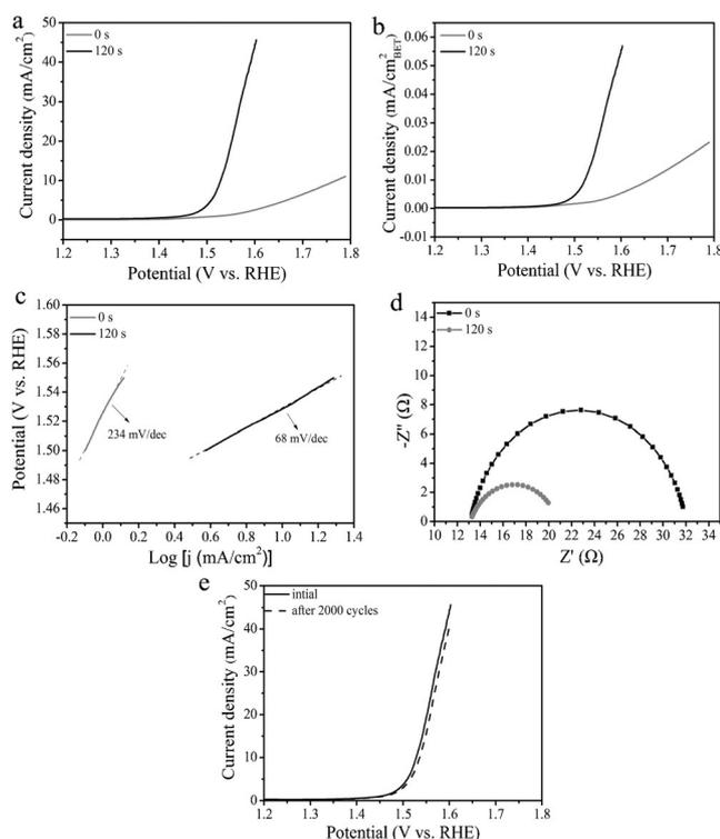
**Figure 4.** a) The polarization curves of OER on pristine  $\text{Co}_3\text{O}_4$  (0 s) and the plasma engraved  $\text{Co}_3\text{O}_4$  (120 s). b) The polarization curves normalized by the BET surface area. c) Tafel plots and d) Nyquist plots of OER on pristine  $\text{Co}_3\text{O}_4$  and the plasma engraved  $\text{Co}_3\text{O}_4$ . e) Stability of the plasma-engraved  $\text{Co}_3\text{O}_4$  after 2000 cycles.
