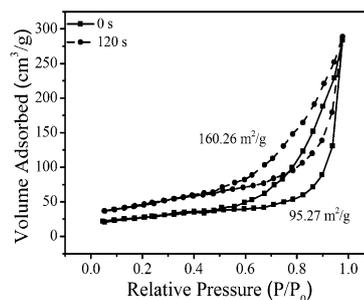
**Figure 2.**  $\text{N}_2$  sorption isotherms of pristine and plasma-engraved  $\text{Co}_3\text{O}_4$ .
