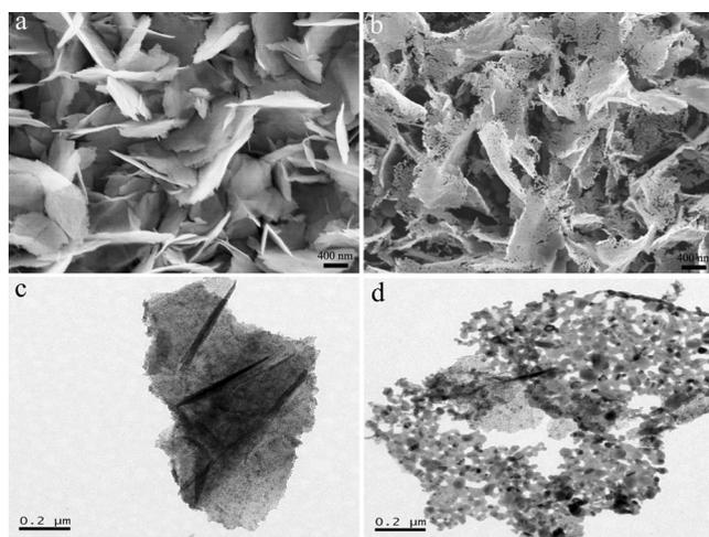
**Figure 1.** SEM images of a) pristine  $\text{Co}_3\text{O}_4$  and b) Ar-plasma engraved  $\text{Co}_3\text{O}_4$ . TEM images of c) pristine  $\text{Co}_3\text{O}_4$  and d) Ar-plasma engraved  $\text{Co}_3\text{O}_4$ .
