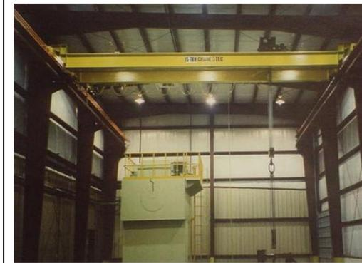
A load lifting system consisting of a hoist which moves laterally on a beam, girder or bridge which in turn moves longitudinally on a runway made of beams and rails. Loads can be moved to any point within a rectangle formed by the bridge span and runway length.
