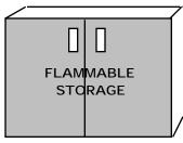
• Small quantities of flammable liquids should be stored in ventilated steel storage cabinets.
