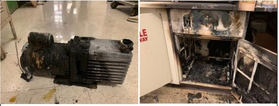
The student was alone in the lab at 6:30 PM when he engaged the power switch on the hood to turn on the vacuum pump. He reports that the vacuum monitor on the rotary evaporator indicated that the pump was not supplying vacuum, so he turned off the power switch. When he flipped the switch back on, he heard "a loud bang" and saw the cabinet door "burst open." The vacuum pump was on fire, producing orange flames and black smoke.
