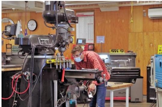
Milling is the process of removing material from a workpiece by feeding it into a rotating cutter at a chosen direction. When using a manual mill the operator turns handles that feed the workpiece into the rotating cutter along the X, Y, and Z axes. The process of milling can shave down surfaces, cut pockets, cut angled chamfers and drill holes.
