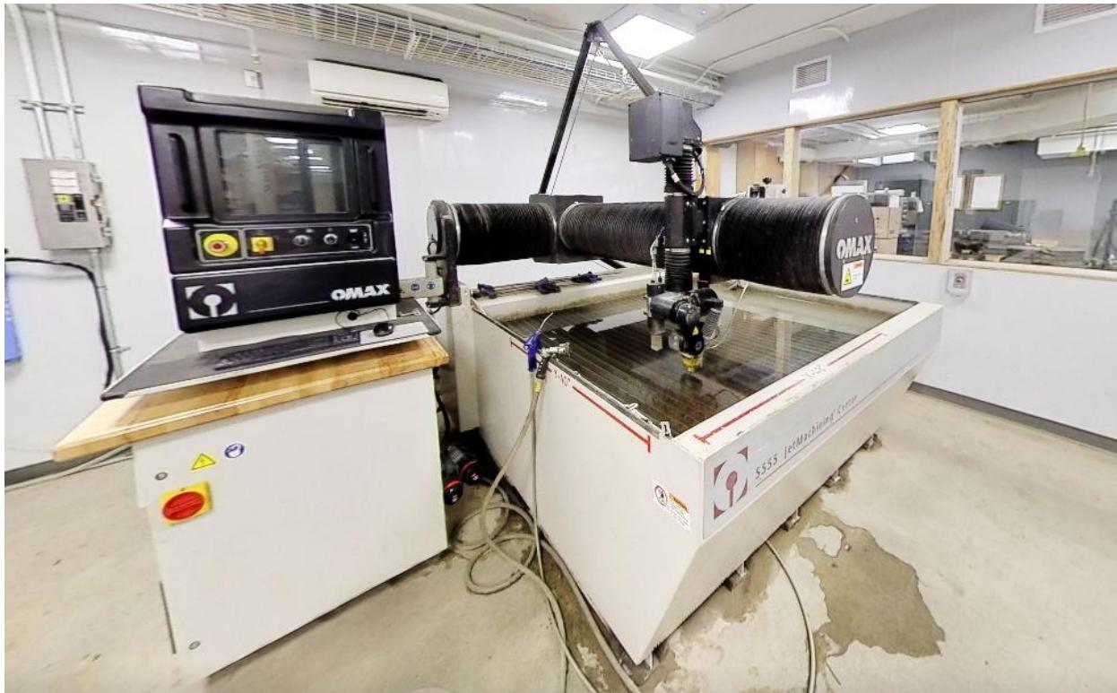
A waterjet cutter uses a stream of water pressurized and forced through a small nozzle to cut materials. For harder materials, fine abrasive particles (commonly garnet) are mixed with the water stream, creating a high-velocity slurry that can cut metals, stone, glass, and composites with extreme precision.
