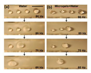
FIG. 3. (Color online) Optical images of the water droplets with and without a microgel on nanofilm coated half-pipes. A 5  $\mu$ L droplet moves from right to left collecting three 2  $\mu$ L droplets without (a) and with (b) microgels. As the drop volume gets larger the frequency of vibration is lowered to transport droplets. Three microgels were sequentially transported and merged into a single droplet on the nanofilm. (scale bar: 5 mm).
