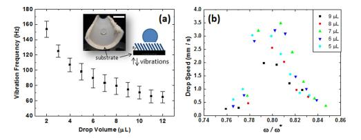
different frequencies and drop volume cluster around the same peak, which indicate that the velocity peaks are due to resonance effects arising from the matching of the vibrational and natural frequencies.<sup>15</sup>
