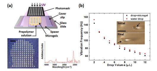
FIG. 2. (Color online) (a) Schematic of microgel synthesis, FTIR of the microgel, and optical image of fabricated microgels are shown (scale bar in the inset is 1 mm). (b) Vibration frequency of as a function of water droplet size with and without a microgel encapsulated within the transported droplet. The inset shows a microgel encapsulated by 5  $\mu$ l water drop, vibrated at 94 Hz on directional nanofilm (scale bar: 5 mm).
