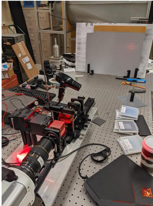
**Fig. 2** Picture of the compact, self-aligning focusing schlieren system in the FPI lab at CWRU.
