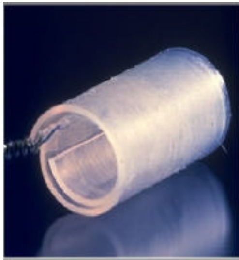
Fig. 9. Photograph of the self-sizing spiral cuff electrode. The spiral configuration can open or close to accommodate a range of different diameter nerves.
