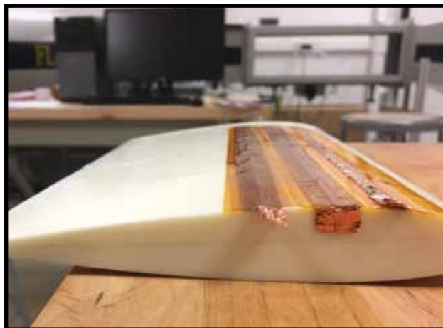
Ghosh's prototype of the dielectric barrier discharge plasma actuator tape.
