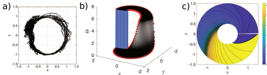
FIG. 4.3. *Noisy Stuart–Landau oscillator with  $y$ -polarized noise* given by (4.4) with  $\omega = 1.99$ ,  $\kappa = 1$ , and  $\sigma = 0.2$ . Example trajectory (a) ( $\Delta t = 0.01$ , trajectories generated in polar  $(r, \theta)$  coordinates and then converted to Cartesian  $(x, y)$  for analysis), MRT phase  $\Theta(x, y)$  (b), and its contour lines, i.e., isochores of the MRT phase (c). For the parameters used,  $\bar{T} = 20.93$ .
