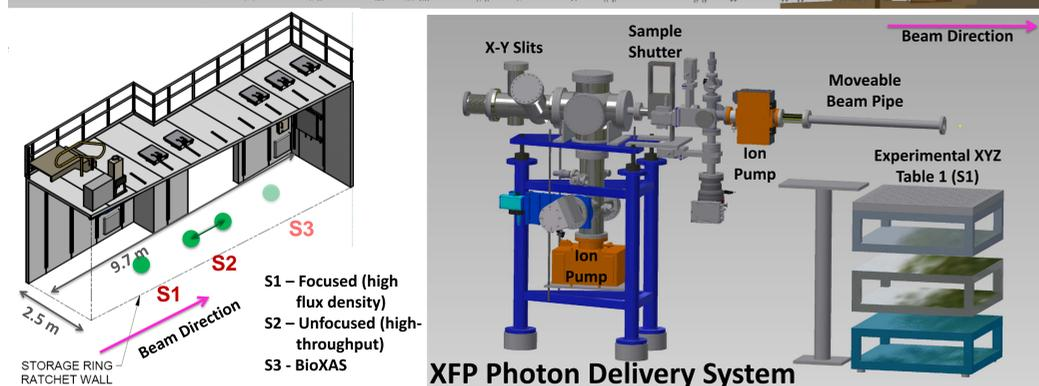
The XFP beamline (NSLS-II 17-BM) delivers focused (single focusing mirror inside the shield wall) white beam to several sample locations and endstations in the experimental hut. A sample preparation area is located proximal to the beamline. Construction of the BioXAS endstation is expected to begin Summer 2017.
