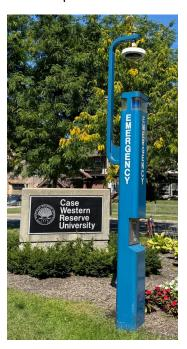
mounted blue light phones. Both phone types have an emergency button and a call button. With a touch of a button, the caller is immediately connected to CWRU's 24-hour public safety dispatch center. The
