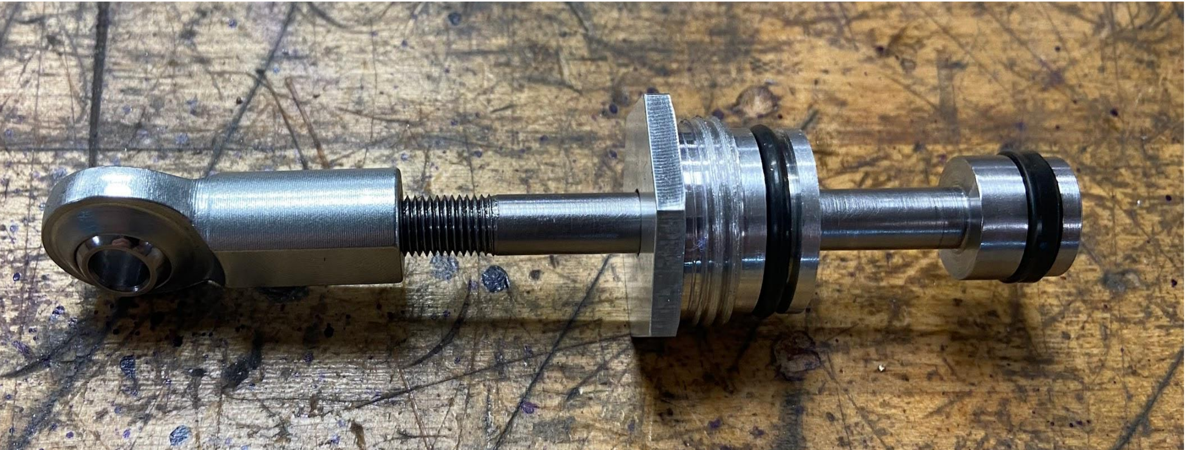
Fig. 11: Images of manual manufactured components. The manual components were manufactured in Sears Think[box] using a manual lathe and manual milling machine. Both components had tight tolerance and surface finish considerations that made machining additionally difficult. The entire assembly will include the 2 manual lathe components, 1 cnc lathe component, as well as seals, springs, and bearings.
