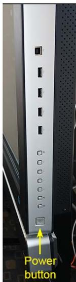
If not, use the monitor's power button. It may be located on the front where the **power light** is located or on its **right side**. Controls vary between displays.
