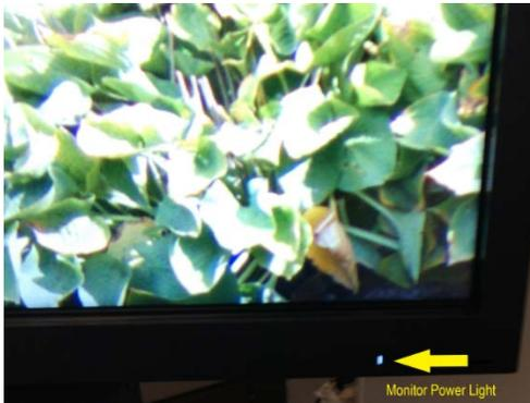
Is it plugged in and the power light on the monitor lit? Every display has a power light showing if there is power to the system and the monitor is on.
