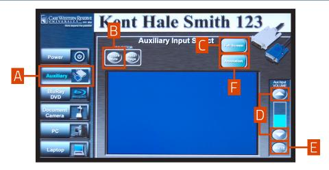
Select the **Auxiliary [A]** button if you are using (1) equipment such as a digital camcorder or video game console or (2) VCRs available via special request. The images from the auxiliary device will be displayed on the screen.
