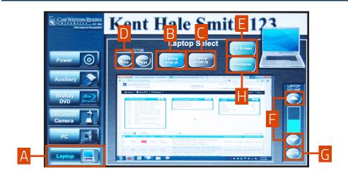
Select the **Laptop** option [A] to display the desktop of a laptop connected to the TEC system with the projector.
