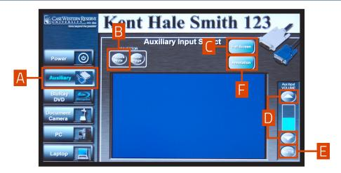
Select the **Auxiliary [A]** button if you are using (1) equipment such as a digital camcorder or video game console or (2) VCRs available via special request. The images from the auxiliary device will be displayed on the screen.
